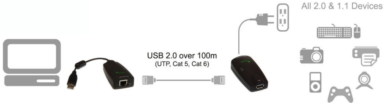
USB extension up to 100m Cat 5e cable
