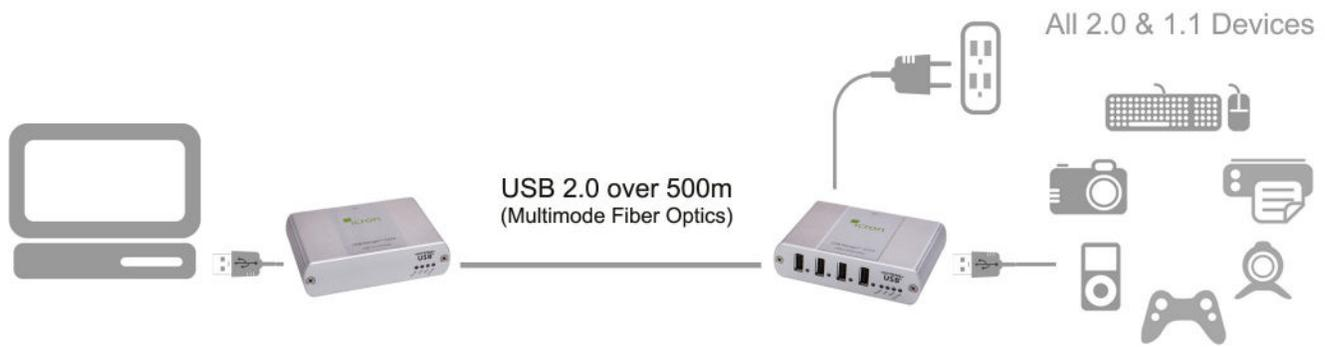
USB extension up to 500m over fiber optic cable
